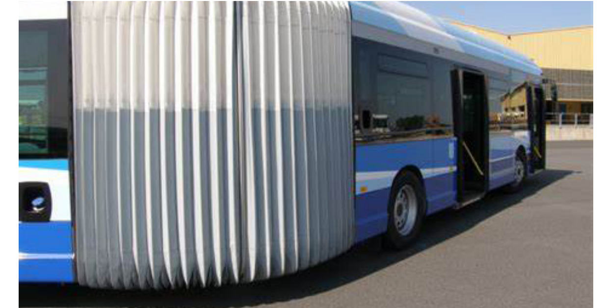
Bus Bellows designed with ROSTA DR ®
