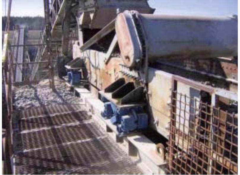
Fig. 1: Linear vibrating screening machine on ROSTA AB's in a very high steel-structure plant.
