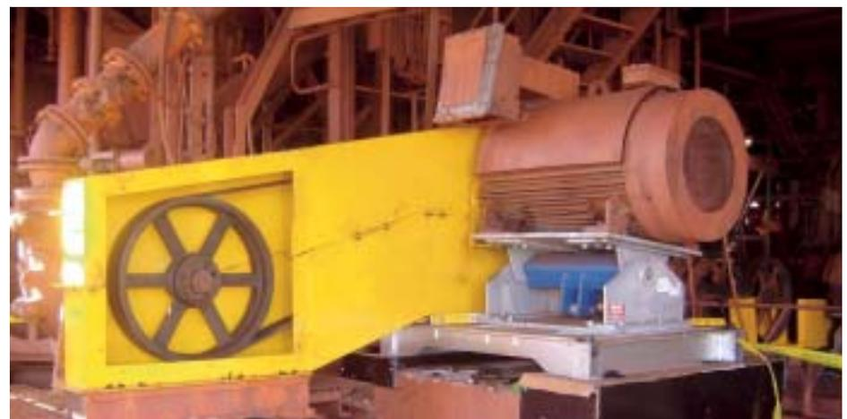
ROSTA motor base type MB 100 with 220 kW drive motor for a **Warman** centrifugal pump (Photo: BHP Billiton-Mining, Australia)
