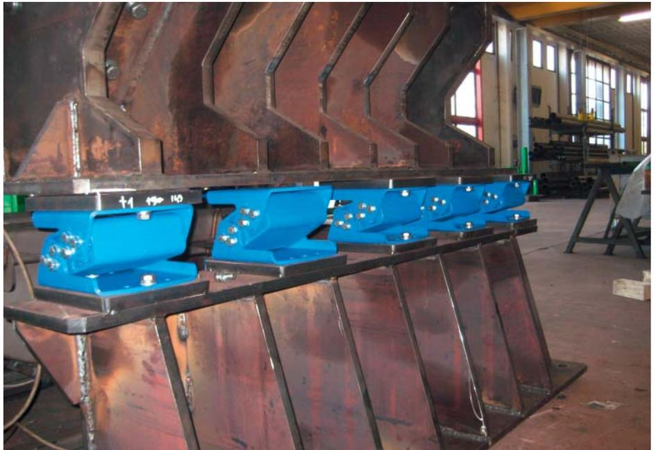
Detail showing a hammer mill mount; thanks to the high deflection capacity of these vibration dampers, practically no reactive forces can be measured on the machine sub-frame.
