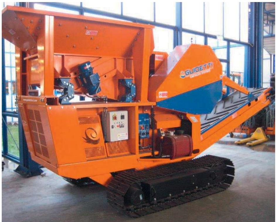
„Caesar Junior“ mobile building rubble crusher with a two cubic metre material bunker mounted on four ROSTA AB-D 50 oscillating mountings.
