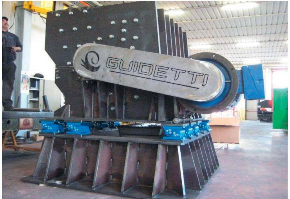
*Guidetti hammer mill („tearing wolf“) for larger objects, such as office machines and televisions, mounted on ROSTA ESL 50-2 anti-vibration mounts to absorb high levels of reaction forces.*
