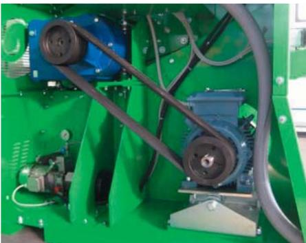
*Drive motor for the belt drive on a shredder shaft: maintenance-free mounting on the ROSTA MB 38 Motorbase.*
