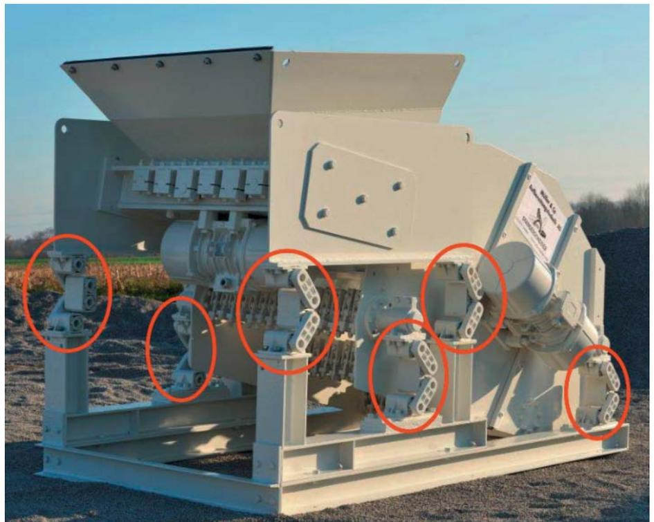
Feed-end with pre-screener and subsequent bar classifier; both are mounted on ROSTA AB-HD 50-2 screen mounts.
