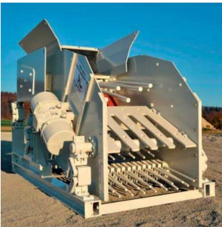
Discharge-end of the Mueller classifier with cascading bars and separator grid.
