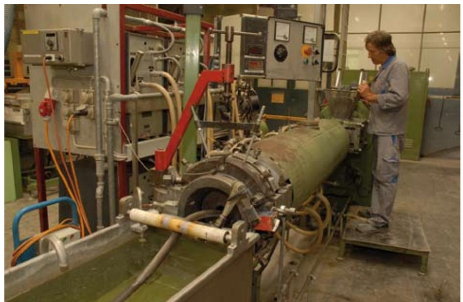
*Extrusion of the ROSTA rubber profiles*
