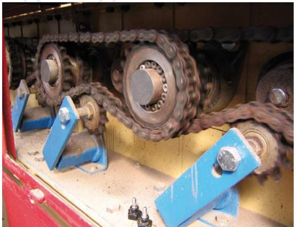
Elastic chain tensioners on an infeed section
