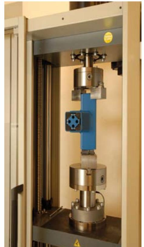
*Torque testing machine in the ROSTA laboratory*
