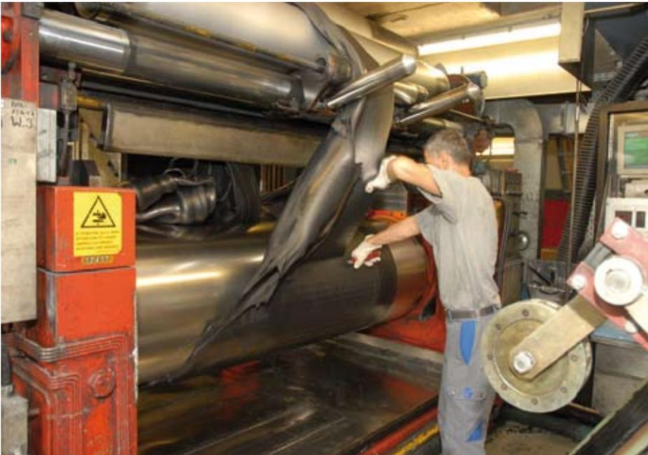
*Discharge masticator for rubber mixtures*
