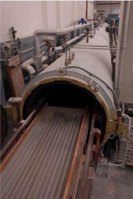
*Vulcanisation in steam-heated autoclave*
